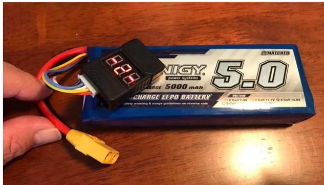
Be aware that the damaged cell may loose charge during storage, regularly check the balance of the battery, and top-up as needed.
